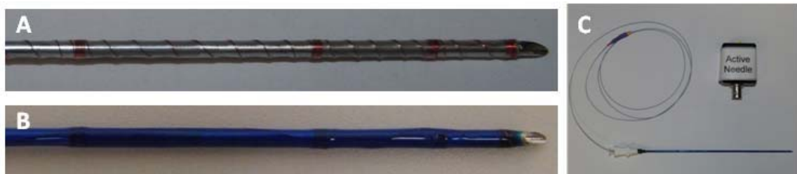
Figure 3.2.1. Active needle with close up of tip uncovered (A) and covered (B). Needle with coaxial extension and circuit box seen in (C).
