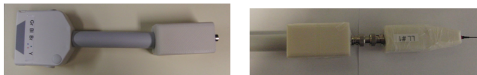
Figure 4.2.8. Flexible adapter to preamplifier with guidewire handle to eliminate coaxial cable extension.
