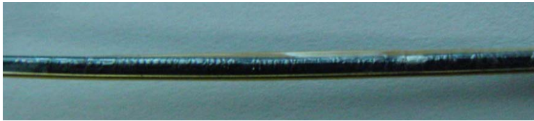
Figure 4.3.3. Guidewire shaft with two polyimide ports placed on either side to measure external heating profile.
